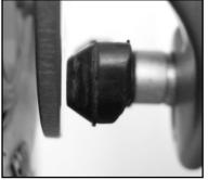
2. Loosen CABLE SCREW so the cable can be pulled to adjust the gap between brake pads and the rotor.
