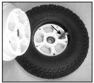
4. Remove top half of hub then flip tire and tube over so valve stem points down.
