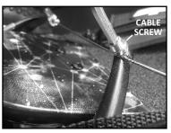
2. Lay brake cable into the groove in the top of the right brake arm and tighten brake CABLE SCREW a little.
