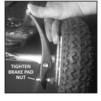
Tip: To prevent brake pad from moving press hard against the top of the brake arm to hold the brake pad in place while tightening the brake pad nut.
